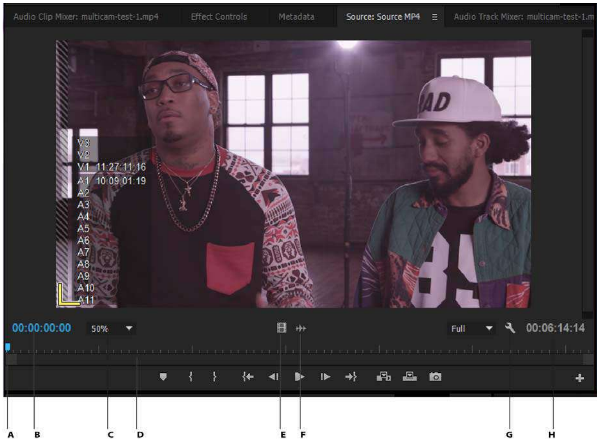
A Playhead B TimeCode C Scaling options D Zoom scroll bar E Drag video F Drag audio G Settings button H In/Out Duration
