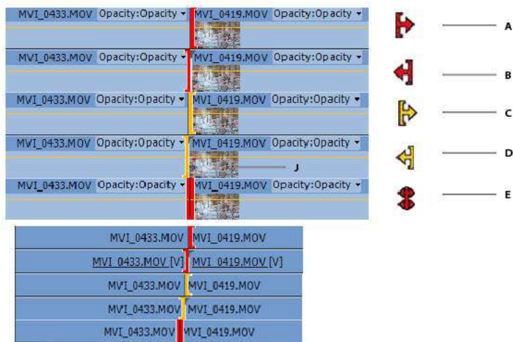
A Regular Edit cursor B Regular Edit cursor C Ripple Edit cursor D Ripple Edit Cursor E Rolling Edit Cursor
